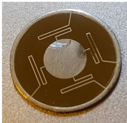
Ni based \mu -fluidic chips on \text{CaF}_2 window
